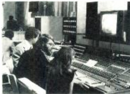
Rupert Neve demonstrated their automated console system with provision for synchronization of audio and video tracks. Monitor shows status of video track.
