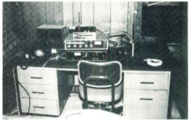
Equipment set up at Decatur airport to receive signal from parachutist and relay it toward Dallas.
